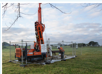
Figure 2 Drilling rig used to collect core samples. The rig may be supported by a four-wheel drive ute and a truck with a water bowser covering an area of approximately 15m 2
